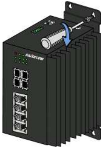
Figure 4-5 Installing the wall-mount plane on the wall
