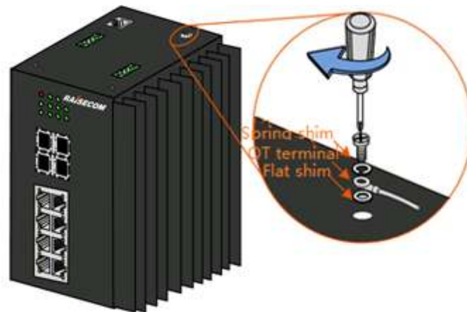
Figure 4-7 Connecting the grounding cable
